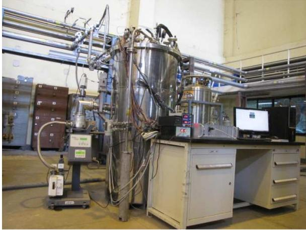
Figure 8 The Closed Loop Heat Exchanger Experimental Test Facility
