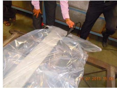
Figure 5 PFHE Being Leak Tested for Global External Leak Using Sniffer Probe (Hood Method) Method of MSLD
