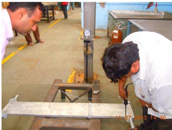
Figure 4 PFHE Being Leak Tested with Sniffer Probe Method of MSLD
