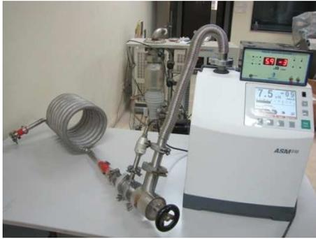
Figure 6 The Helical Coil Being Leak Tested
