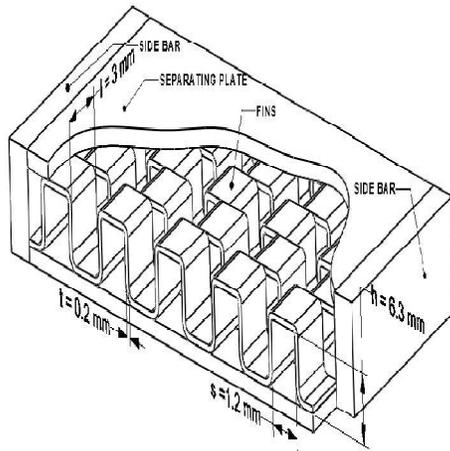
Figure 2 Schematic of OSF used in the developed PFHEs
